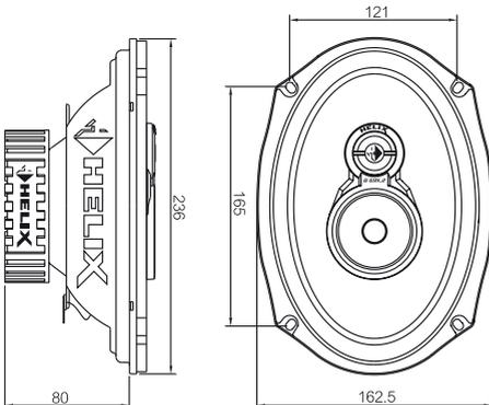
\*Alle Abmessungen in mm
