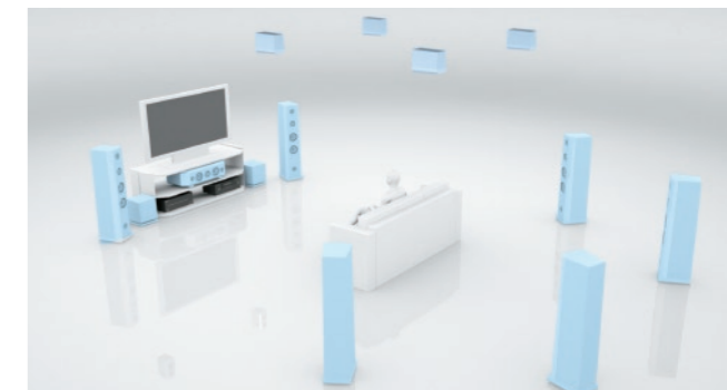
Speaker Layout Example of a Dolby Atmos Home Cinema (7.2.4ch)
