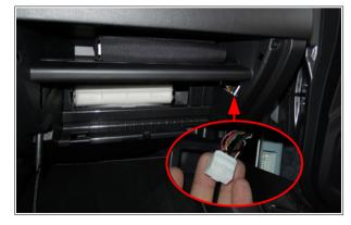
6 Disconnect the Bluetooth interface located under the OEM unit.
