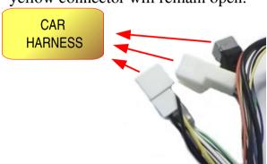
3 Connect the ISO to the radio harness and bushings for services.
