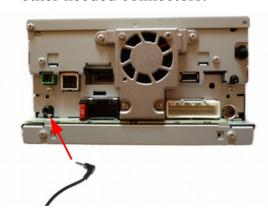
5 If the OEM head unit is DAB ready, unplug the DAB connector behind the glovebox.
