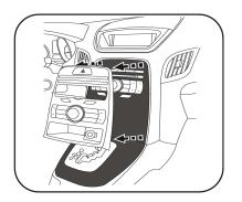
Unclip and remove the radio/climate control trim panel
