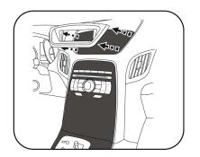
4. Unclip and remove the display trim panel above radio.
