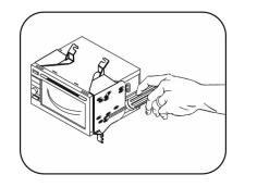
8. Attach the Dobule DIN bracktes to the Pioneer unit, connect the wiring harness.
