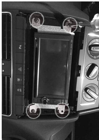
Connect all cables, insert the AFT unit into the housing and fix it with the screws; verify the proper functioning of the system, including the touch buttons on the facia plate.
