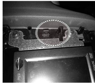
Before to place the AFT unit into the housing, cut and remove the two pivots per side, as shown in the picture.
