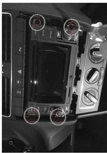
Remove the OEM head unit by unscrewing the four screws circled.
