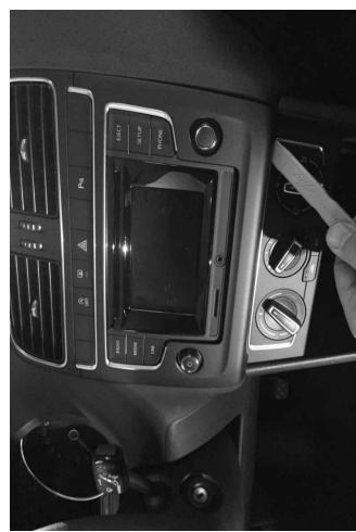
In the picture the original dashboard. Carefully unclip the original panel.
