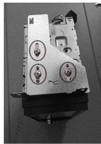
Take the left and right brackets and mount them on the AFT unit using the screws supplied.
