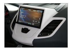
Mount the Pioneer head unit to the Double DIN facia plate
