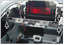
5. Remove the middle bar (cut at the position marked with arrows)
