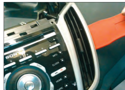
13. Unclip air vents Remove air vents
