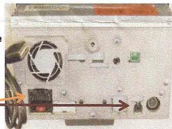
Parking Brake is generated by speedsignal ( Screen off > 8km/h)
