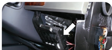
1E TouaregGP (Facelift) Location: Attached to panel as pictured with double-sided tape and cable ties.
