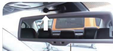
2B Passat 3C, Passat CC Location: Attached to rear view mirror support cover.
