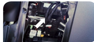
1H Skoda Superb Location: Mounted on dash support cross brace, behind driver side pocket.
