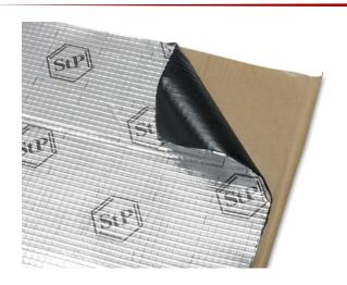
Multicomponent polymer based on butyl rubber supplemented with anticorrosive excipients. The material is a resinous construction of black color with the adhesive layer covered with corrugated aluminum foil of golden color with black printing and small cell stamping. The adhesive layer is covered with the antiadhesive paper to prevent contamination of material before its applying.
