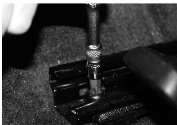
N°5. Unscrew with a "torx 45" tool
