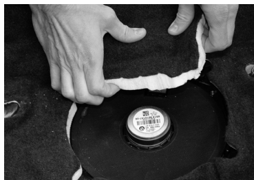
N°15. Raise the carpet to have an access to connector
