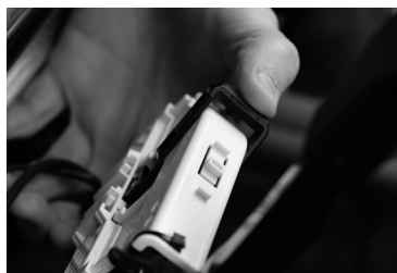
N°9. Unlock the power connector (under the seat)*
