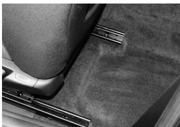
N°3. "Rear" screws to remove the seat
