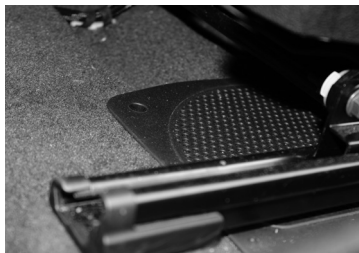
N°1. Subwoofer location (under the front seats)
