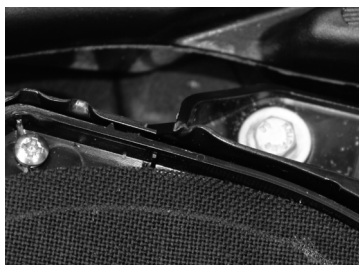
N°18. In case of the original subwoofer is glued, unscrew the 2 CHC screw (to remove the complete enclosure)
