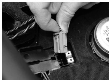
N°17. Disconnect the factory plug to terminal
