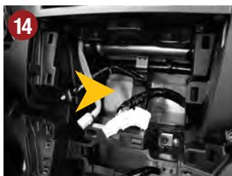
14.) Lay the connection cable sets of new ESX device (refer to page 4-5) inside the vehicle to the desired location.
