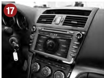
17. Before you complete the installation of the new ESX device, check its function. Please note that it may take up to 15 minutes, until a GPS signal can be received (in the open). After the successful check of the functions, re-assemble the new device in the reverse order (steps 1-12).
