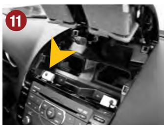
11.) Flip the ventilation unit upwards
