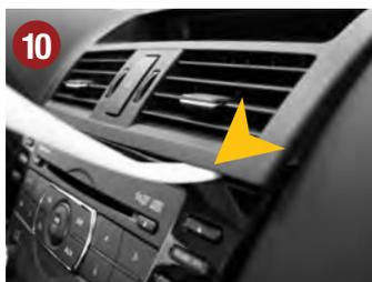
10.) Loosen the panel of the ventilation unit.
