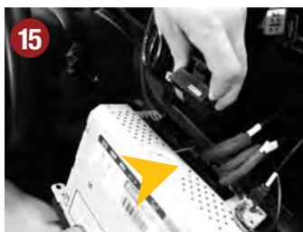
15.) Now connect all connections these according (refer to page 4-5) with the sockets on the new ESX device. Plug in also the car specific and the antenna connector.
