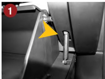
1.) Unlock the damper of the glove box and carefully flap down the glove box.
