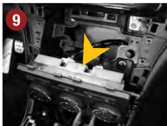
9.) Pull out the AC controller unit and let it hang out of the bay.
