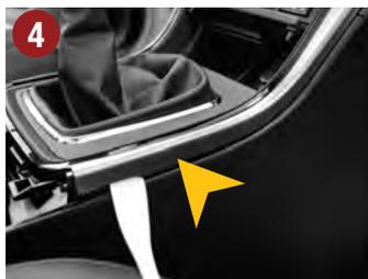
4.) Loosen the decoration panel of the center console on each side.
