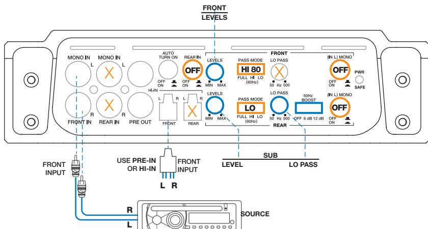
Using also REAR INPUTS to drive SUBWOOFER:
