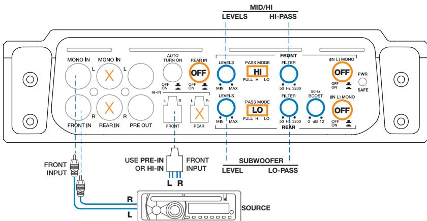
Using also REAR INPUTS to drive SUBWOOFER:
