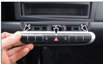
2. Remove the switch unit (fixed by clamps) by pulling it towards you
