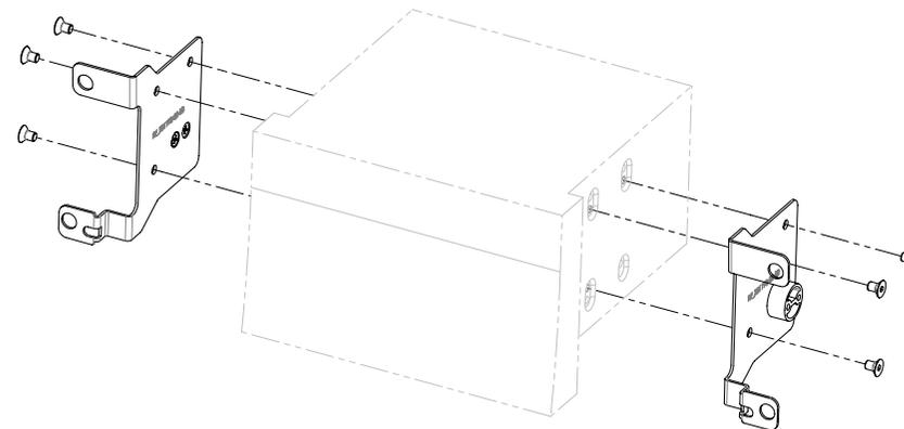
5. Mount mounting brackets left and right to INE-W928R Connect all required circuit points and place the Double DIN head unit on dash board
