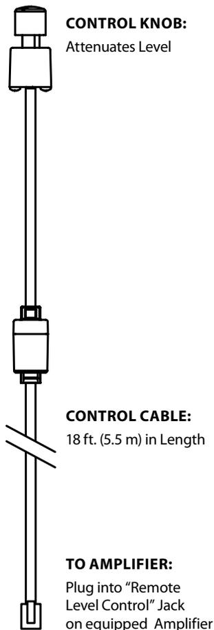
Note: Should a replacement control cable be needed, you can use any standard telephone-to-wall-jack cable with six position terminations. The cable itself can be 2-conductor, 4-conductor or 6 conductor.
