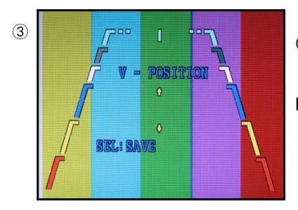
③ On step no.2, once press "SEL" key again, you can move the line vertically by "UP", "Down" keys.
