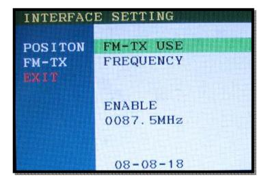
Get the Factory Mode Operated with pressing UP->DOWN->UP->MENU keys of t he keypad sequently
