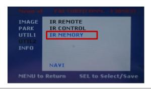
Press ◀ button or UP→DOWN→UP→MENU button of remote to run factory menu and then choose UTIL2→ IR MEMORY→NAVI
