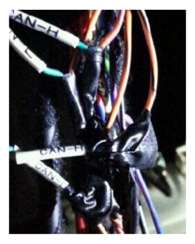
User can find original CAN wires behind air conditioner controls
