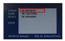
First of all, press ◀ button on remote controller 2 seconds long or press UP→DOWN→UP→MENU button in order to access Factory mode. Choose IR MEMORY on I-DRV.
