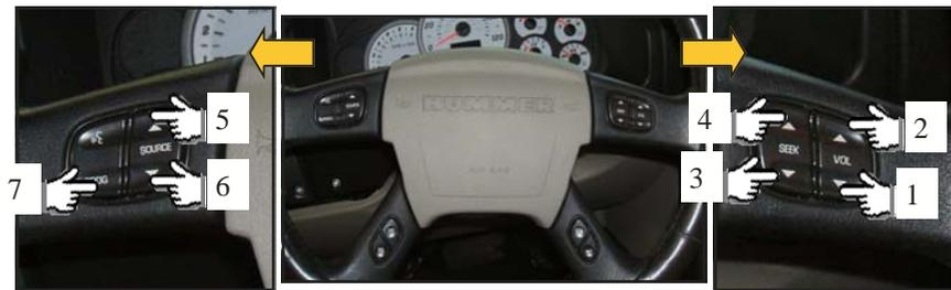
Once assigned the 7 functions, press 3 times the UNICOM button. **The LED will light GREEN.**
