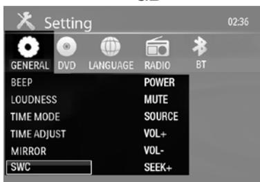
By pressing **SWC**, a window will appear showing a number of available command. Use the arrow-keys to move to the requested command. Press to store the selected command and wait for it to enlighten the icon, this operation must be carried out for all available commands on the steering wheel.
