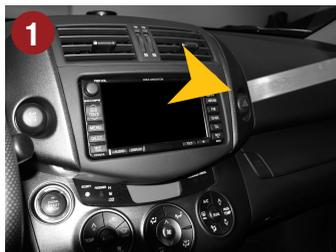
1.) Remove carefully both decoration panels on the right and left of the radio panel with mounting wedges.
