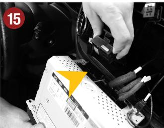
15.) Lay the connection cable sets of new ESX device (refer to page 4-5) inside the vehicle to the desired location and connect these according with the sockets on the new ESX device. Plug in also the huge car specific and the antenna connector. For a proper connection of the both Fakra jacks you need an additional adaptor (refer to page 2)
