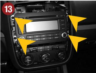
13.) Remove the 4 screws (Torx 25) which hold the radio.
