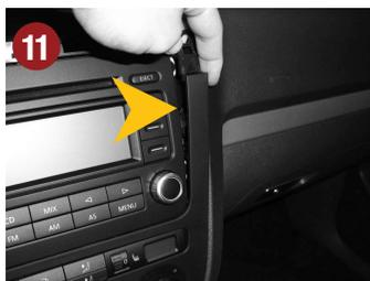
11.) Carefully remove the panel around the radio.
