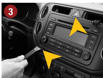
3.) Carefully pry the radio panel from the dashboard with a mounting wedge. Then remove the connector of the warning light switch in the middle.
