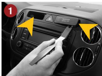
1.) Remove the 2 panels over the original radio with a mounting wedge.
