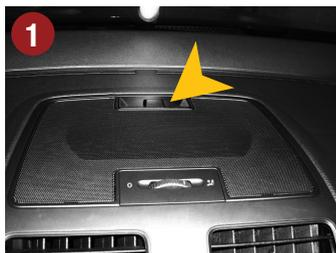
1.) Remove the light sensor from the ventilation grille (depending on model, if applicable) below the windscreen.
