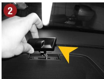
2.) Lift the sensor carefully, after you have slightly loosen the left and right fixings. Then disconnect the cable connector, but make sure that the connector slips not inside.
