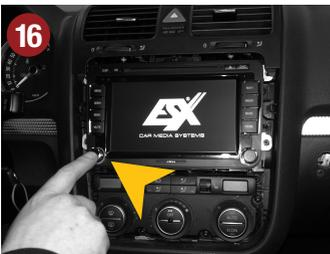
16. Before you complete the installation of the new ESX device, check its function. Please note that it may take up to 15 minutes, until a GPS signal can be received (in the open). After the successful check of the functions, re-assemble the new device in the reverse order (steps 1-13).
