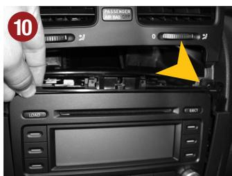
10.) Remove both screws of the panel and loose the radio slightly.
