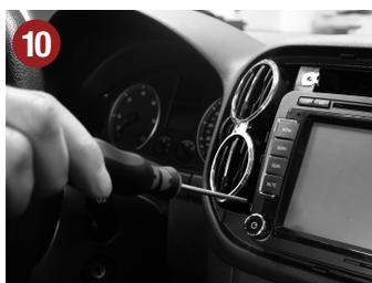
10.) After the successful check of the functions, re-assemble the new device in the reverse order (steps 1-5).
