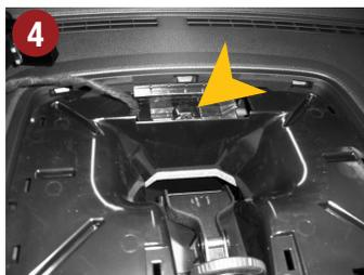
4.) Remove the fixing screw of the ventilation cover.
