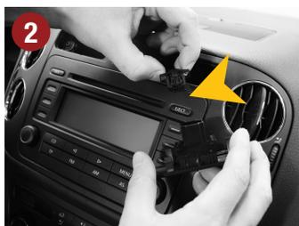
2.) Disconnect the cable plug on the right panel (Airbag Control Lamp) on the back.
