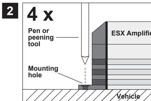
Keep the amplifier at the chosen mounting location in the vehicle.
