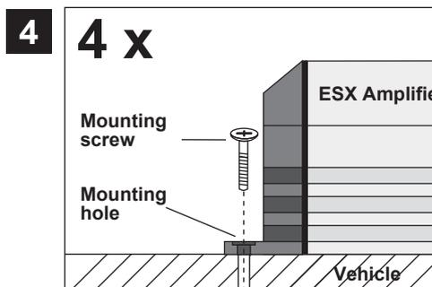
Then uphold the amplifier to the chosen position and fix the screws through the mounting holes into the drilled screwholes.
