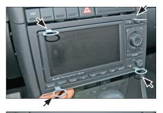
Use 4 radio release keys to dismount the OEM radio.
