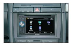
Connect alle required circuit points and push the double DIN head unit until it snaps in.
