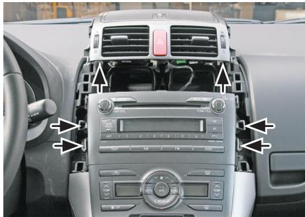
2. Pull up the air vent / hazard switch unit.
