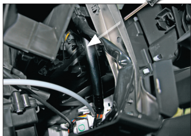
Remove locknut from head unit (driver's side underneath the dashboard). Place the screw driver BEHIND the frame as shown on the picture
