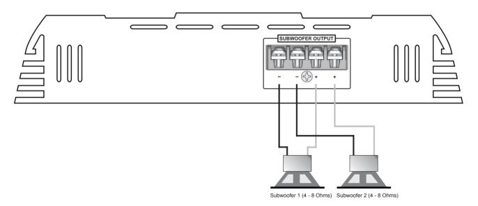
**CAUTION:** Ensure by any means, that the total impedance load of subwoofer is not lower than 2 ohms. Too low impedance cause high temperature and will shut down the amplifier operation.
