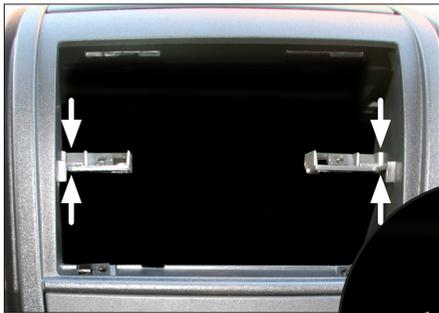
2. Cut away original brackets (marked with arrows) with appropriate tools to clear space
