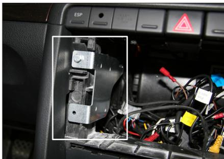
3. Place mounting frames as positioning help in order to mark the plastic areas that have to be cut away
