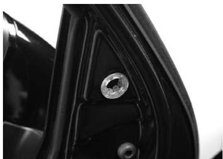
Place the rubber washer onto the door frame.
