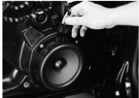
Assemble the Focal speaker using the rivets provided with the kit.
