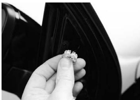
Remove the rubber washer from the tweeter mounting.
