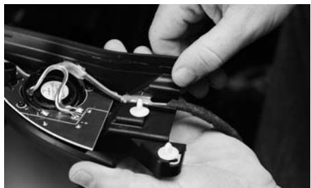
Place the two plastic clips onto the Focal tweeter mounting.
