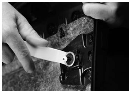
Put the fasteners in the "unlock" position before reassembling the door panel.
