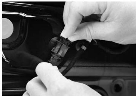
Reassemble the Focal tweeter mounting and reconnect (equipped with VW connector).
