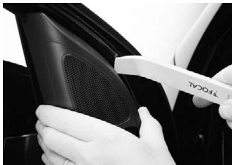
Dismantle the original tweeter mounting (using the Focal tool provided).
