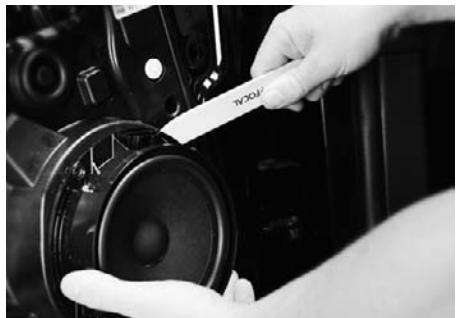
Drill out the original rivets (x4 per woofer).
