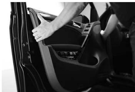
Dismantle the door panel (using the FOCAL tool provided).
