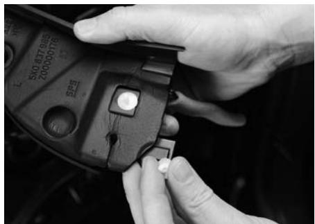
Remove the two plastic clips from the original part.
