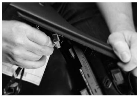
Disconnect the connector plugs (window switches, multiplexer, outside rear-view mirror...).
