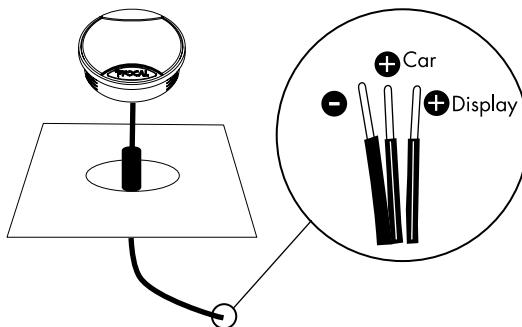
When installing on a demonstration display, connect the "display" wire.
