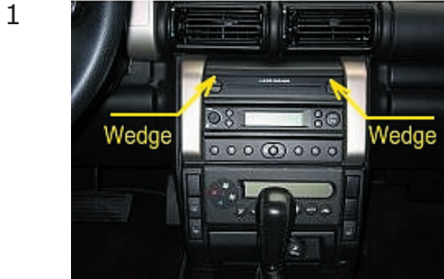
Car is equipped with original head unit. Remove plastic cover with wedge
