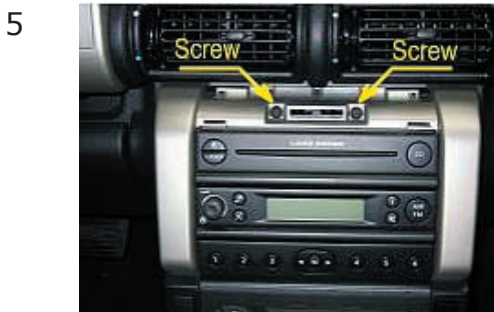
Remove 2 screws at the location of the arrows. Remove storage bin.
