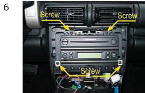
Remove 4 screws at the location of the arrows. Remove Head unit
