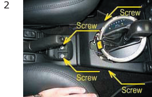
Remove 4 screws at the location of the arrows.
