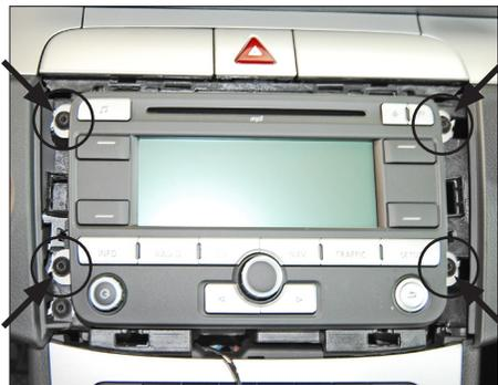
2. Remove the 4 Torx (TX20) screws (These screws will be used again later).
