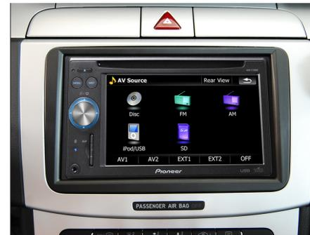
6. Connect all wires and fix the Pioneer Double DIN head unit with original Torx (TX20) screws
