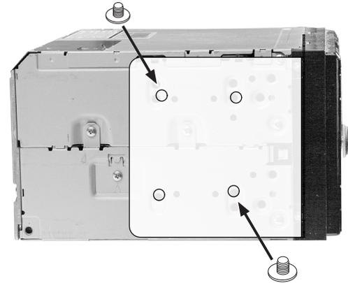
5. Push the Pioneer Double DIN head unit into the fascia plate and fix the sides of the head unit with 2 screws on each side.
