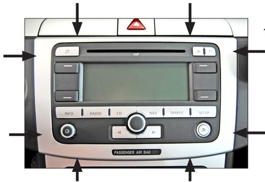
1. Remove the original trim frame, surrounding the radio (fixed by clips).
