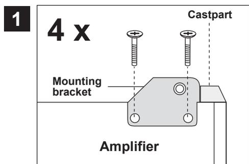
Before mounting the brackets you can remove the castparts on each end. Then install the 4 supplied mounting brackets on the bottom side of the amplifier with the supplied screws. Ensure that the angled side of the brackets are pointed to the inner side. The pre-drilled screw holes are located on each corner of the amplifier.
