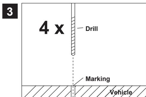
Put the amplifier aside and then drill the holes for the mounting screws at the before marked locations. Please ensure not to damage any components of the vehicle while drilling the holes. Alternatively (depends on the material of the surface) you can also use self-tapping screws.
