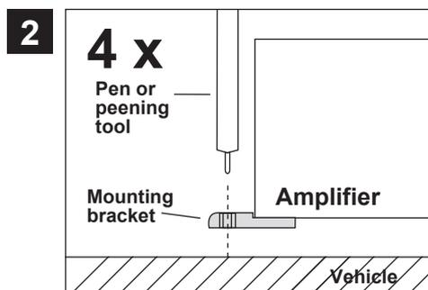
Uphold the amplifier with the mounted brackets to the chosen mounting location in the vehicle. Then mark the four drill holes with a appropriate pen or peening tool and lead through the designated holes of the mounting brackets. Attend that there remains enough space for the installation of the cables and ensure that they will not be bended and have sufficient pull relief.
