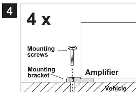
Then uphold the amplifier to the chosen position and fix the screws through the holes of the mounting brackets into the drilled screwholes. Ensure that the mounted amplifier is fixed tight and not get loosen. Then mount the maybe before removed castparts again to the device.
