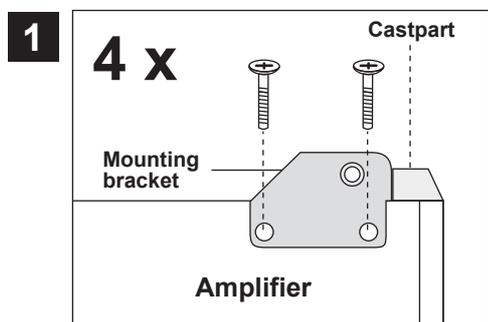
Before mounting the brackets you should remove the castparts on each end. Then install the 4 supplied mounting brackets on the bottom side of the amplifier with the supplied screws. Ensure that the angled side of the brackets are pointed to the inner side. The pre-drilled screw holes are located on each corner of the amplifier.
