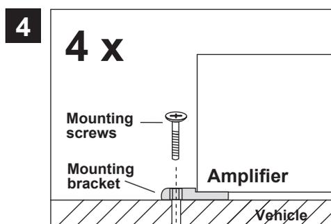
Then uphold the amplifier to the chosen position and fix the screws through the holes of the mounting brackets into the drilled screwholes. Ensure that the mounted amplifier is fixed tight and not get loosen. Then mount the before removed castparts again to the device.
