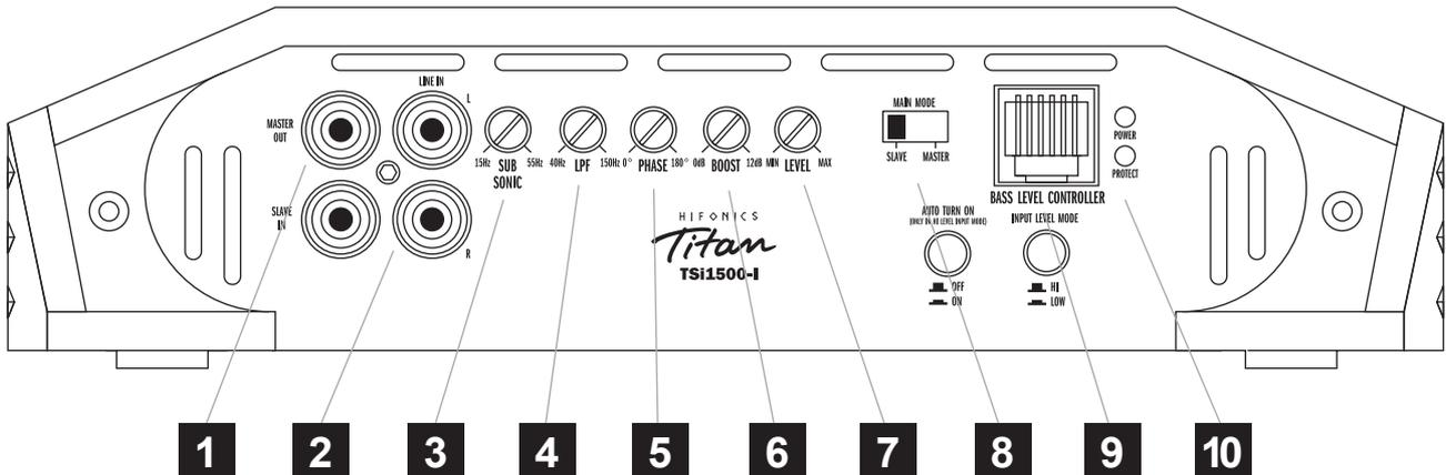
**1** The **SLAVE IN/ MASTER OUT RCA jacks** are suitable to connect an additional identical built amplifier in MASTER/SLAVE mode. Please check the chapter **Interconnection Example: MASTER/SLAVE** on page 22.
