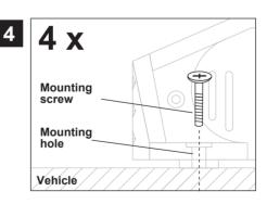
Then uphold the amplifier to the chosen position and fix the screws through the mounting holes into the drilled screwholes.
