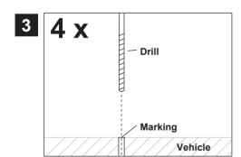
Put the amplifier aside and then drill the holes for the mounting screws at the before marked locations.
