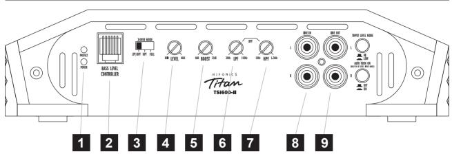
POWER/PROTECT (Also located on the supplied Bass Level Controller)
