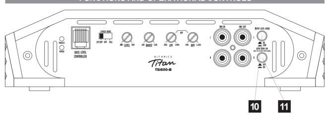
The INPUT LEVEL MODE switch sets the operation mode of the LINE IN RCA connectors. In pushed position (LOW), the LINE IN is suited for pre-amplifier signal (low level signals, pre-amplifier outputs from the head unit). In the non-pushed position (HI) the LINE IN connectors are suited for high level signals from the speaker outputs of the headunit.
