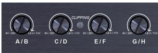
To start now with the adjustment of the first channels (A and B) turn the left control knob slowly clockwise until the green clipping LED lights up red. At this point turn the control slowly counterclockwise until the clipping LED lights up green again and then keep this position. Now the channels A/B are adjusted.
