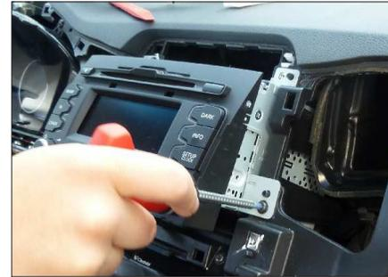
6. Remove screws of OEM head unit
