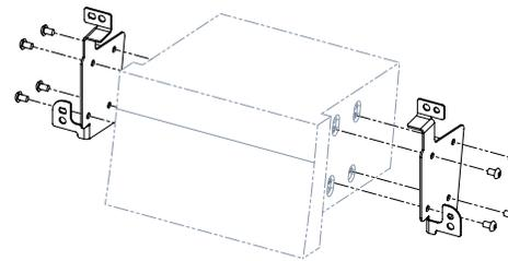
7. Attach metal mounting brackets to Double-DIN Navigation
