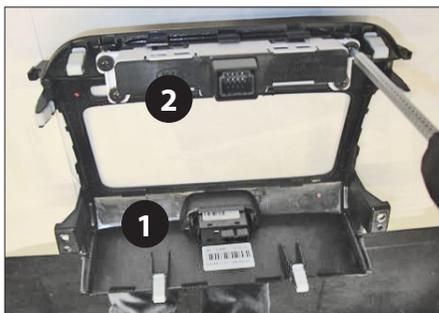
10. Remove hazard light switch (1) from OEM head unit - attach it to double DIN fascia plate
