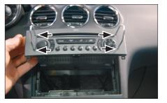
Insert two radio release keys in the openings of the OEM head unit.
