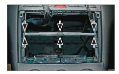
I. Remove middle bar to clear space for the Double DIN head unit.
