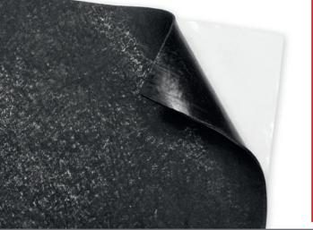
**STP VIZOMAT** – self-adhesive bitumen vibration damping material. It is a multilayer construction made of a sheet on the basis of a bitumen composition and mounting adhesive layer protected with an antiadhesive coating. The working temperature range is from 45°C below zero to 70°C above zero. The material has a high degree of elasticity when heated and is easily mounted to complex surfaces. It needs to be heated by a thermal pistol.
