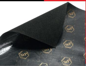
STP BTP 5 GOLD – self-adhesive material based on elastic polyurethane foam 5 thick with an adhesive layer protected by the specific impregnated anti-adhesion film that makes the material water and wear resistant, improves its sound absorbing properties and considerably improves its resistance to the ultraviolent radiation.
