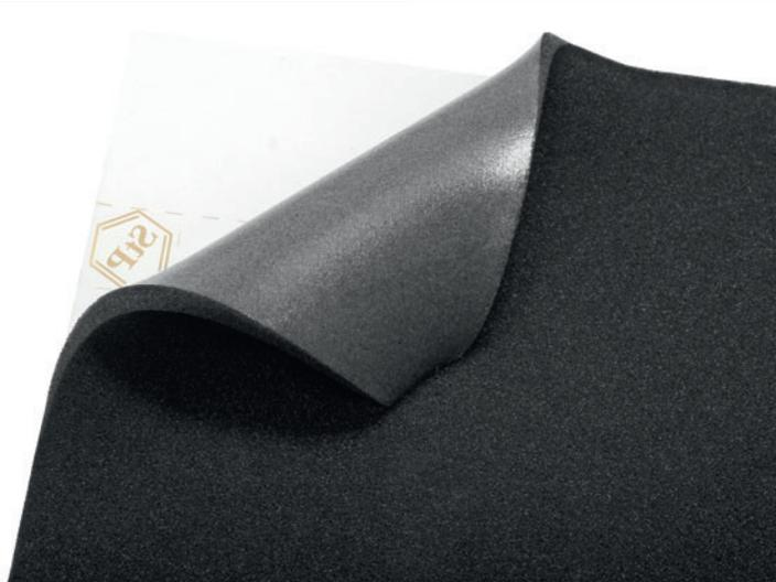
**STP BTP 10 GOLD** – self-adhesive material based on elastic polyurethane foam 10 thick with an adhesive layer protected by the specific impregnated anti-adhesion film that makes the material water and wear resistant, improves its sound absorbing properties and considerably improves its resistance to the ultraviolet radiation.
