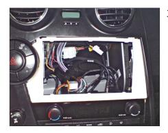
3. Place the new facia plate on the dashboard and fix it with the four screws.
