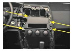
Remove the original bracket, which is fixed by four screws at the location of the arrows.
