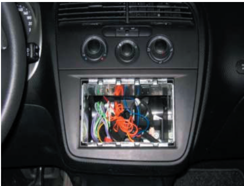
Place 2-DIN metal bracket
