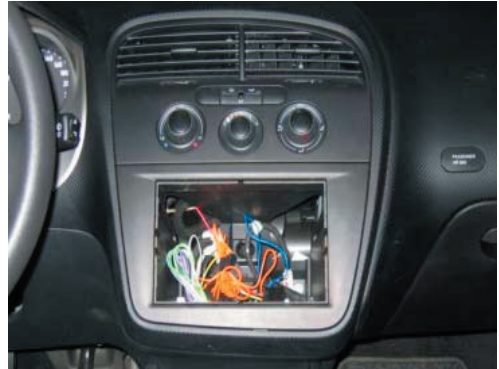
Place replacement panel for Seat.
