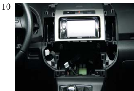
Place the new OEM replacement panel.
