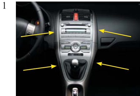
Remove the dashboardpanels around the radio at the location of the arrows.
