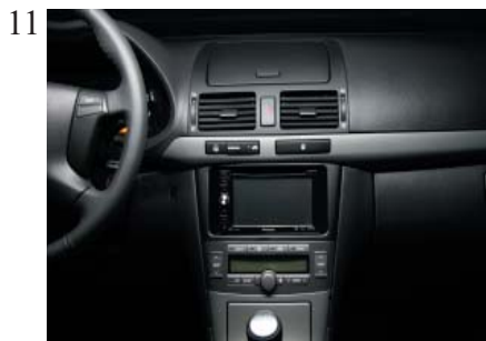
Place the radio trim and replace all dashboardpanels in reverse order.
