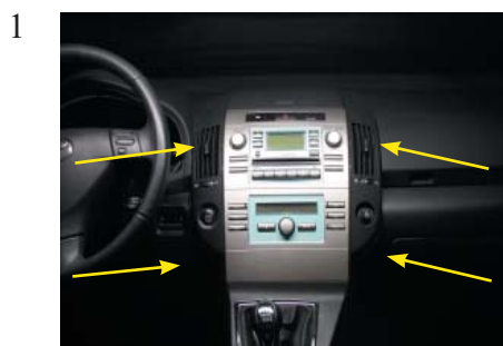
Remove the air shafts at the left and the right side of the OEM radio by using a plastic wedge.
