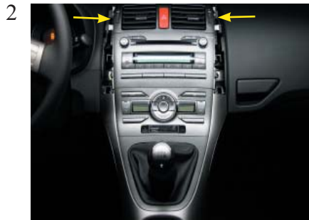
Remove the top air shaft by pulling it forwards.
