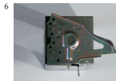
Place the OEM metal brackets on the metal bracket of the new headunit. This will fit into the holes of the metal bracket (if needed mount it with screws).
