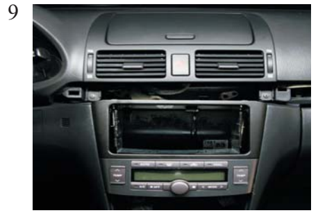
Place the OEM replacement panel with the climate control unit and the metal bracket into the dashboard.
