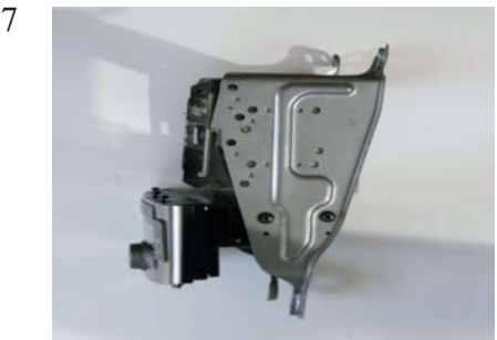
Place the new metal bracket and the climate control unit between the OEM radio brackets. Tighten the climate control with the four original screws.
