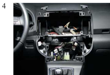
Remove the air shafts at the left and the right side of the OEM radio by using a plastic wedge.
