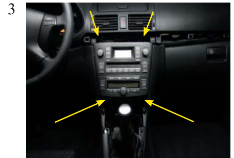
3 Remove the original radio at the location of the arrows. The radio is tighten by four screws.
