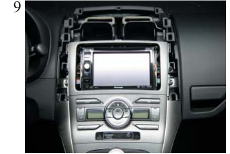
Place the OEM replacement panel.
