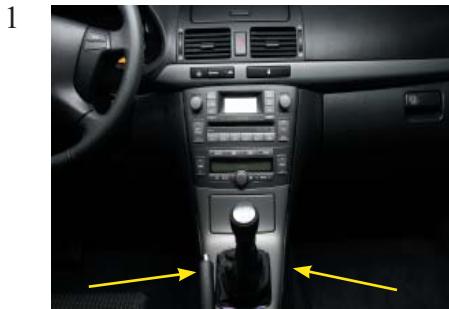
1 Remove the dashboardpanels around the radio at the location of the arrows.
