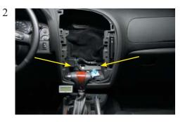
Remove a piece of the plastic panel inside the dashboard at the location of the arrows.(this will give you a beter position of the new headunit)
