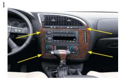
Remove the dashboardpanel around the radio at the location of the arrows. Then remove the orginal radio this is thighten by four screws. Remove the climate control unit.
