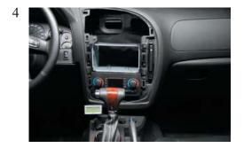
Place the 2-Din metal bracket. Place the climate control unit.
