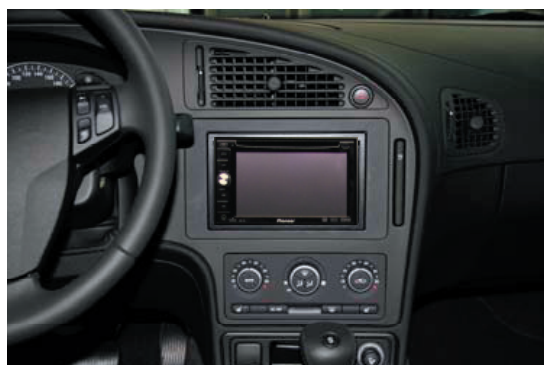
Place the head unit and connect all the wiring.
