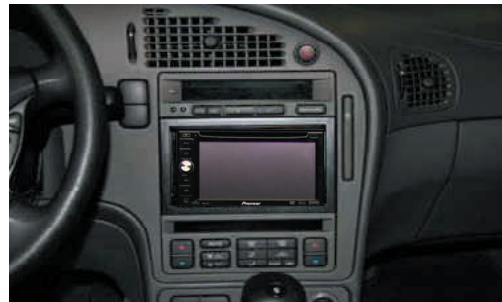
Place the head unit and connect all the wiring.
