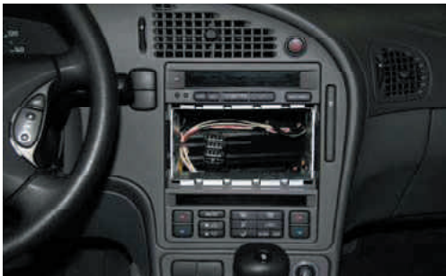
Place the 2-Din metal bracket.
