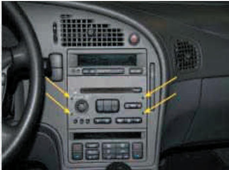
Remove radio using radio removal keys.
