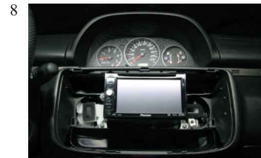
Place the new headunit.
