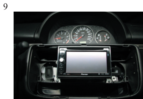
Place the replacement panel.
