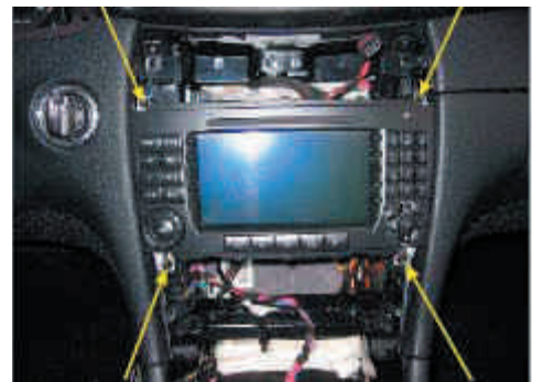
Remove the original radio with a trox 20.
