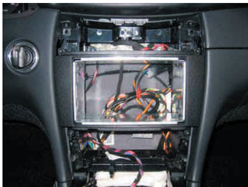
Place the metal 2-din bracket.
