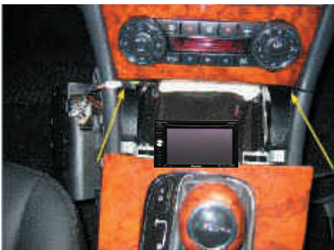
Remove the wooden panel with a torx 20.
