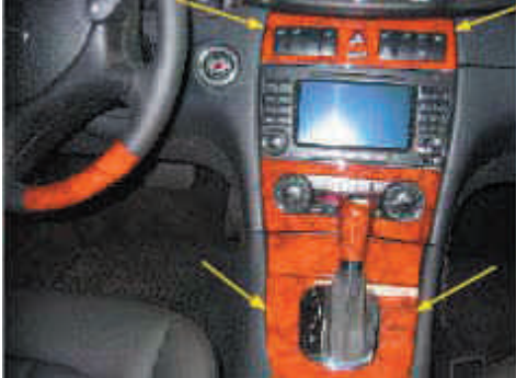
Remove with a plastic wig the wooden panel.
